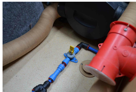
Opening the internal drain valve will empty the majority of the fresh water
