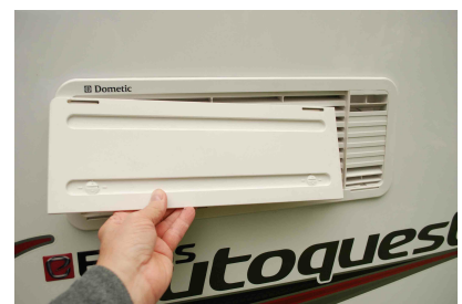
Fit winter covers to fridge exterior vents
