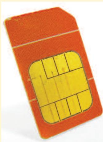
When a SIM is mounted on a card it forms a SIM card. These SIM cards come in a variety of sizes.
