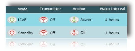
The current unit settings are displayed on the Grid Screen to enable you to see at glance the various modes of your unit. By default, icons will be in their 'Off' state. *Note: The Standby icon does not mean the unit is switched off, just in sleep mode between its set wake-up interval.*
