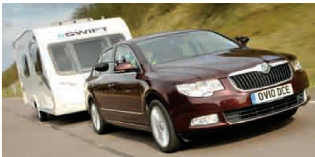
Pushed really hard through the cones for the lane-change test, the Superb 4x4 matched the Superb Estate and BMW X1 and was never pulled off course by the caravan. Only when slowing from 70mph did the AI-Ko ATC system detect the tourer wandering slightly.
