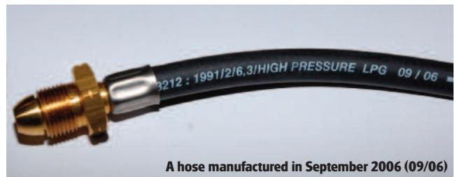
Gas supply hoses deteriorate over time and in use, so they should be replaced at least every five years and more frequently in intensive use conditions. UK hoses will be marked with their date of manufacture and should be inspected frequently for damage and wear.
