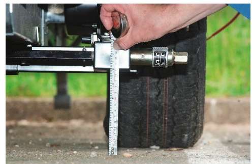
Ground Clearance of 150mm or more is recommended
