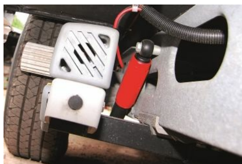
A mover fitted alongside an existing stock absorber
