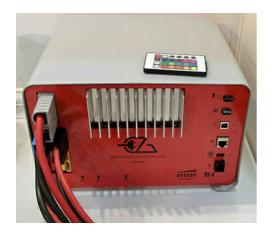
Here we have an inverter and lithium battery combined into one unit. Designed for use with a motorhome, the sockets on the left accept a variety of charging sources including the vehicle's alternator (direct connection) and solar. The battery is rated at 80Ah and the maximum output is 1,500W.
