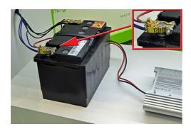
The best advice is to connect directly to the leisure battery via a fuse using clamp type terminals. It is also advisable to keep the DC wiring to the inverter as short as possible to minimise voltage drop, with the associated loss of power. Where long runs are unavoidable you need to compensate by increasing the size of the connecting cables. If in doubt seek professional advice.
