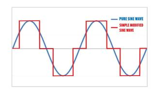
To mitigate these problems you can pay a bit more for an inverter with more steps in the waveform. The drawing here shows a two-step waveform and you can see how much more closely the output matches that of the sine wave. Even so there are still sharp edges that may cause problems with some equipment.
