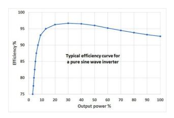
Good quality sine wave inverters can achieve efficiencies of 90-95 per cent in terms of output power to input power. Cheaper modified sine wave variants may be in the range 75-85 per cent. The power loss takes the form of heat generated during conversion and also when in standby.
