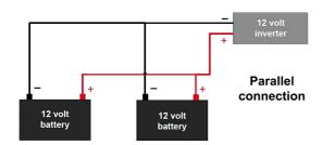
Connecting batteries in parallel (positive to positive, negative to negative) maintains the voltage at 12V while connecting in series (positive to negative) will almost double it to 24V. This latter option only makes sense if you have a 24V inverter.
