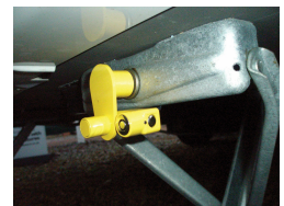
A corner steady lock
