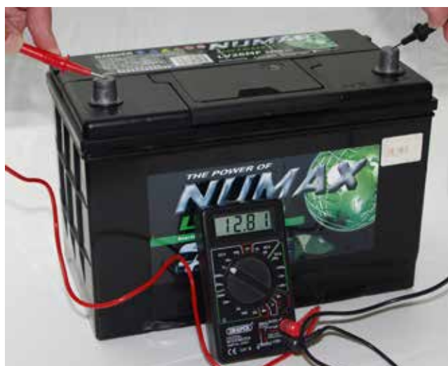
After a day of resting this battery is registering 12.81V, which means it is fully charged
