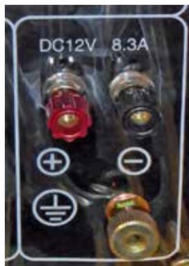
A generator output suitable for battery charging
