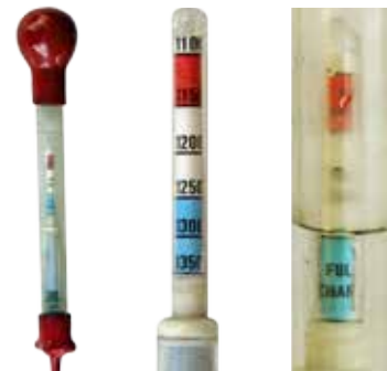
A hydrometer as used for checking the specific gravity of battery acid. The reading shows the battery is close to being fully charged
