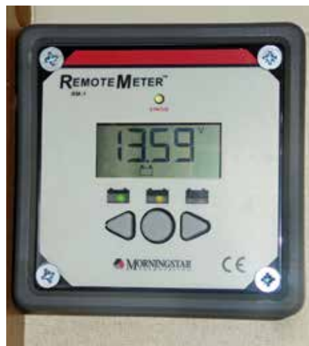
This solar display panel can show voltage, current, amp hours and other information on its screen. It works in conjunction with the PWM charge controller shown below it
