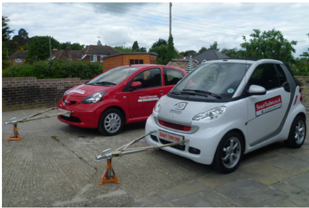
Above: Smart cars fitted with A-frames designed for use with braking systems. Right: A-frame connectors being fitted to the front of a car to be towed.
