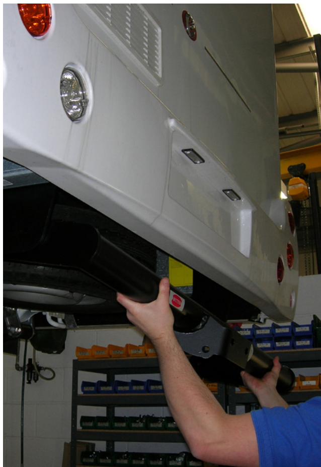
A towbar being fitted to a motorhome
