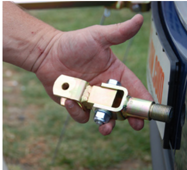
Above: Smart cars fitted with A-frames designed for use with braking systems. Right: A-frame connectors being fitted to the front of a car to be towed.
