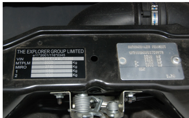
A base vehicle weight plate next to convertor's plate
