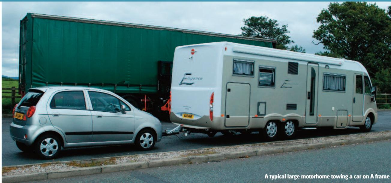
A typical large motorhome towing a car on A frame
