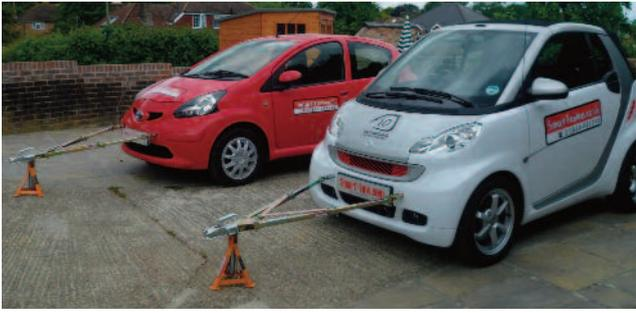
**Above: Smart cars fitted with A-frames designed for use with braking systems. Right: A-frame connectors being fitted to the front of a car to be towed.**
