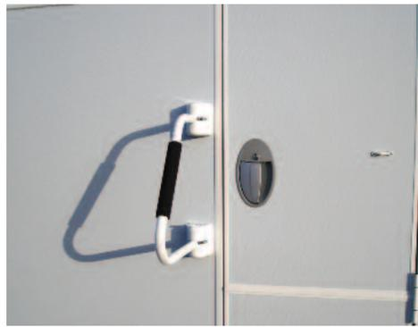
Extra security measures to safeguard your unit include a Shandleo lock (above) that doubles as a hand hold, and a Sleepsafe compact battery window alarm (below)
