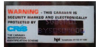
■ **Microchips** – CRiS registered caravans from the 1998 model year have a radio frequency identification (RFID) tag fitted as standard within the bodywork. All previous CRiS registered models can have them fitted retrospectively. Special electronic scanners are available to the police to check for tags and thus identify a caravan, despite efforts of thieves to destroy visible surface identification markings.
