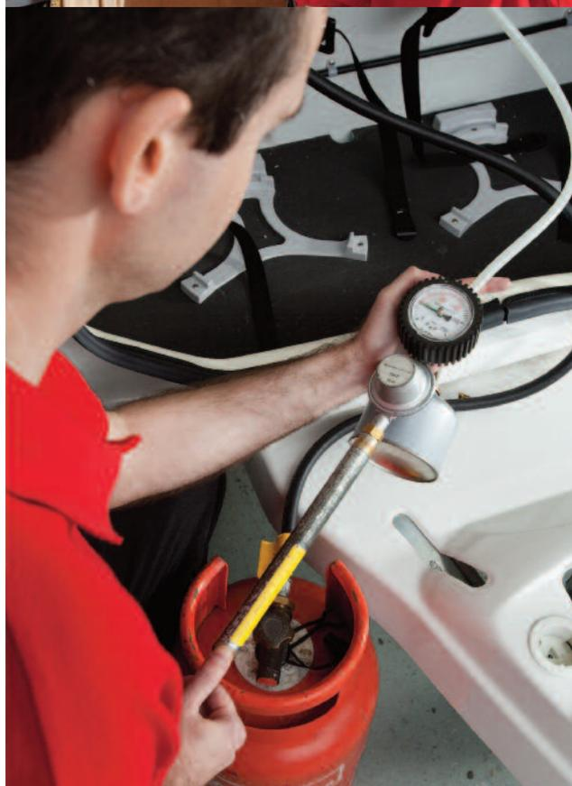
**Pictured from top: Servicing a hitch; checking the fixtures and fittings; gas pressure testing**
