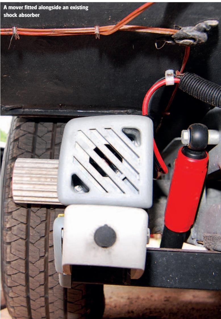
below the chassis at the point of fitting. There's a caravan industry standard recommending a minimum chassis ground clearance of 150mm, so a motor mover with a ground clearance less than this is not ideal.
