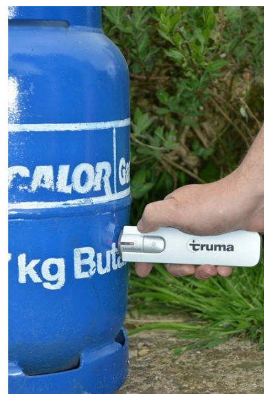
Red indicator on Truma LevelCheck denotes no LPG at that level
