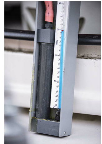
Manometer testing a caravan gas system
